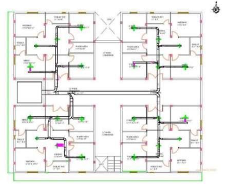
First main duct (supply duct) From AHU to first supply duct =5001.5 Recommended main duct velocity = 1250 fpm So from Macquay duct sizer For rectangular duct width (in inches) = 26 Height (in inches = 24 Equivalent round duct diameter = 27.1 Aspect ratio = 1.08:1
